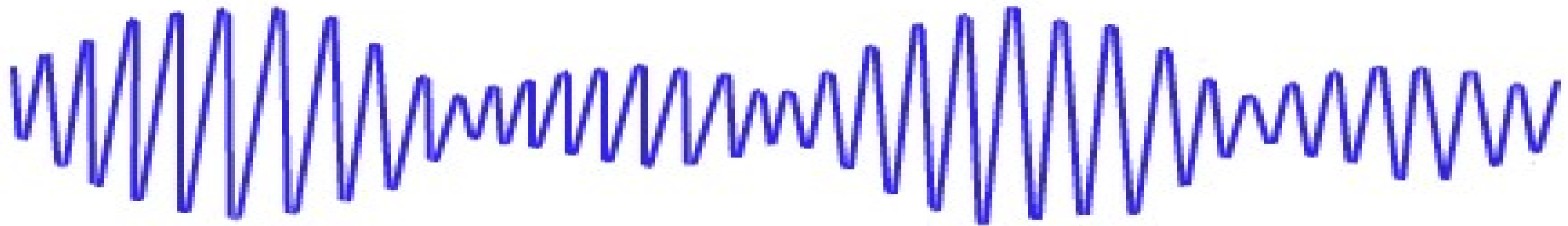
Modulated Carrier Signal
